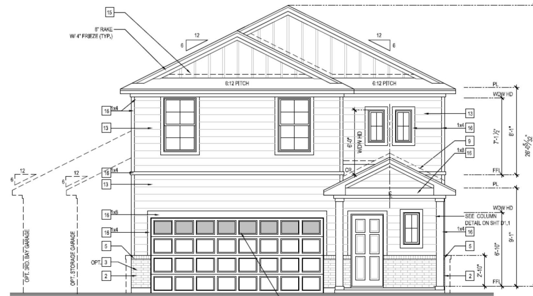
Front Elevation 'B' SCALE: 1/4"=1'-0" AT 22'00" LANDSCAPE 1/8"=1'-0" AT 11'00" LANDSCAPE Front Façade Glazing = 8% (Inc. Eight Glass Inserts in Garage)
