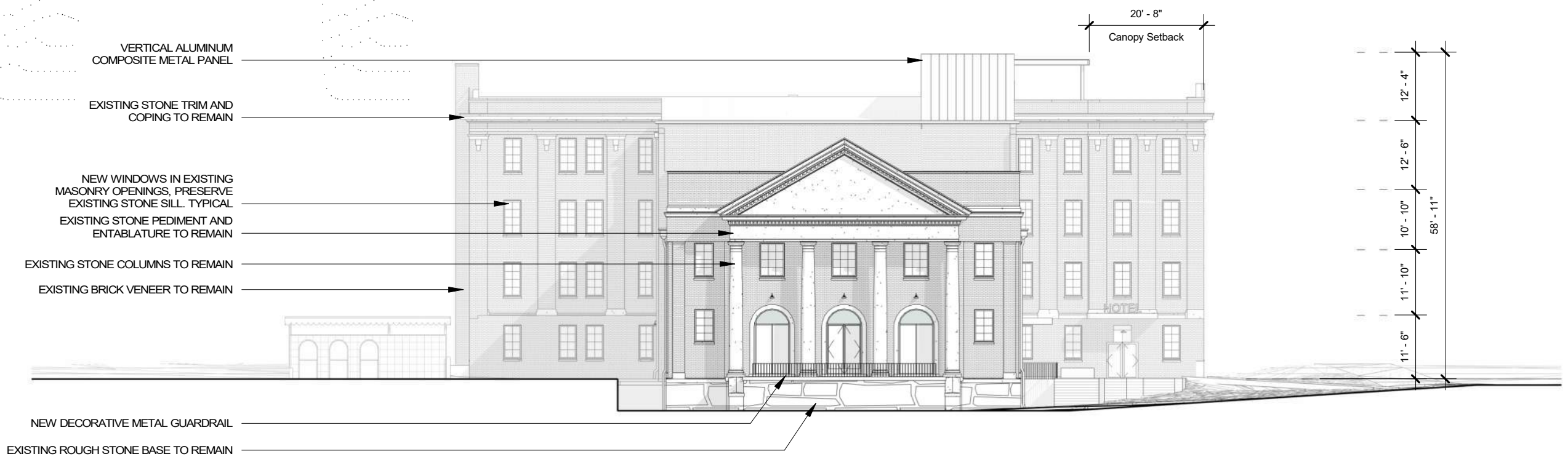
1 WEST ELEVATION - MHZC 3/64" = 1'-0"
