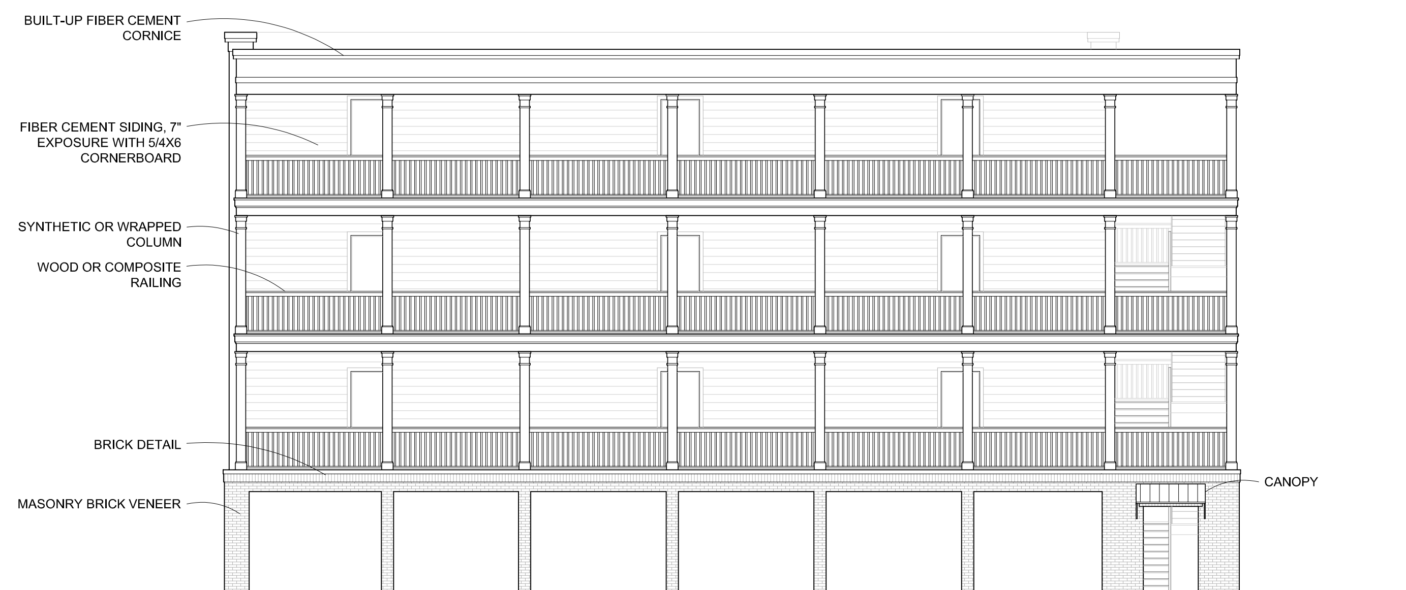
BUILDING 02 REAR ELEVATION - NORTHWEST
