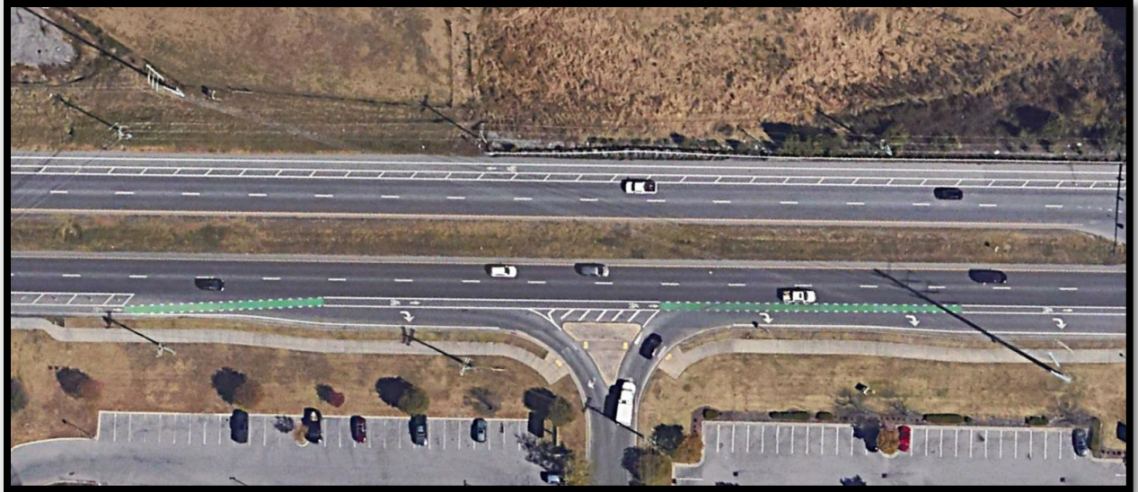
Figure 4-1: Restricted Access Intersecting a Bike Lane on Old Hickory Boulevard (Nashville, TN)
