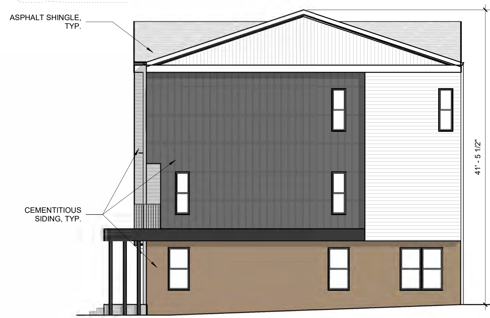
02 BUILDING G - RIGHT ELEVATION
