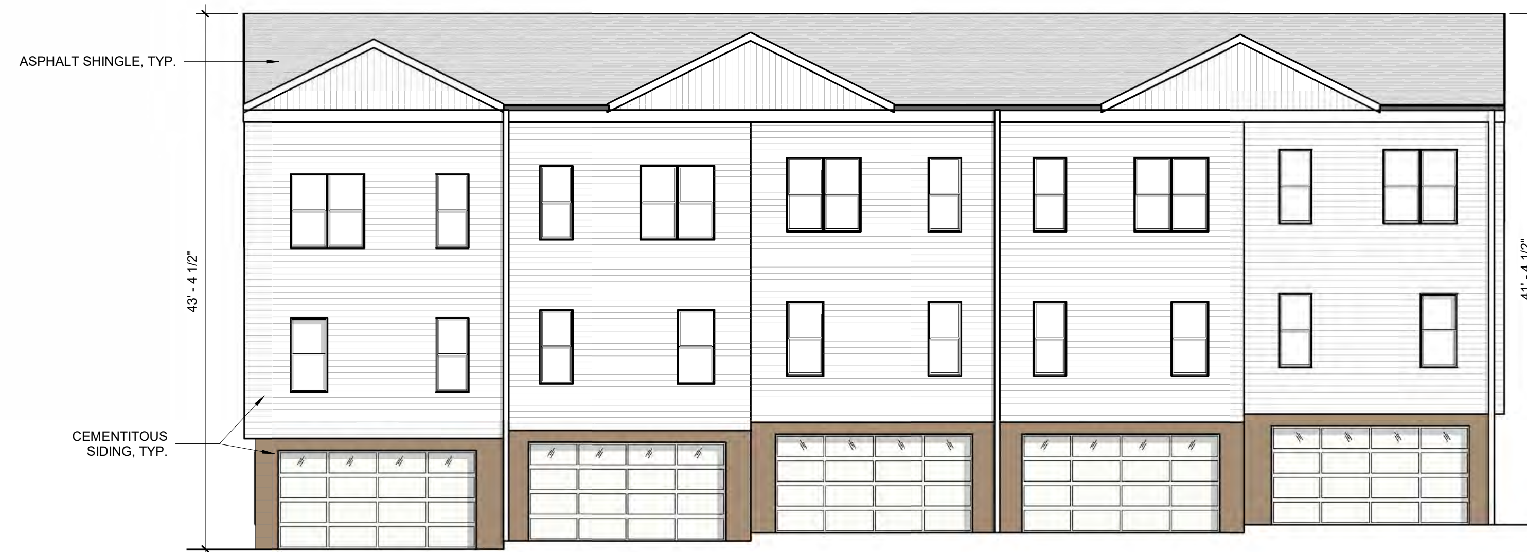
03 BUILDING A - REAR ELEVATION
