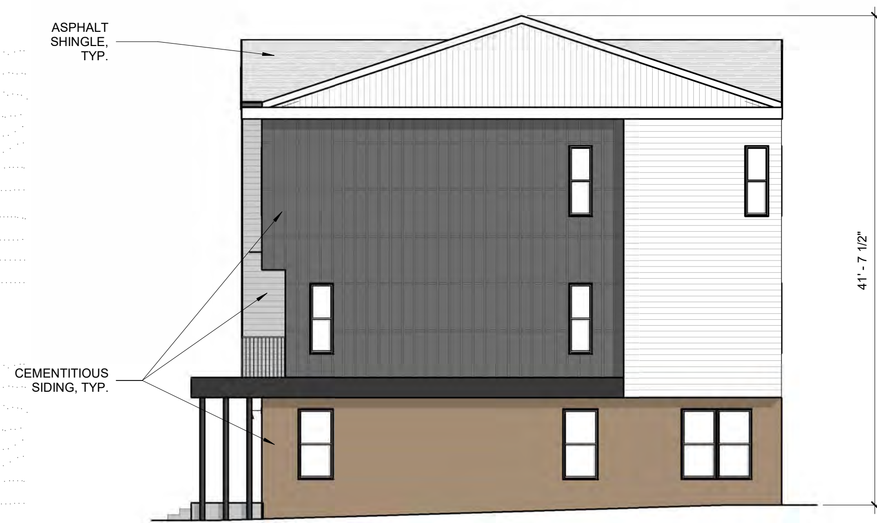
04 BUILDING F - RIGHT ELEVATION
