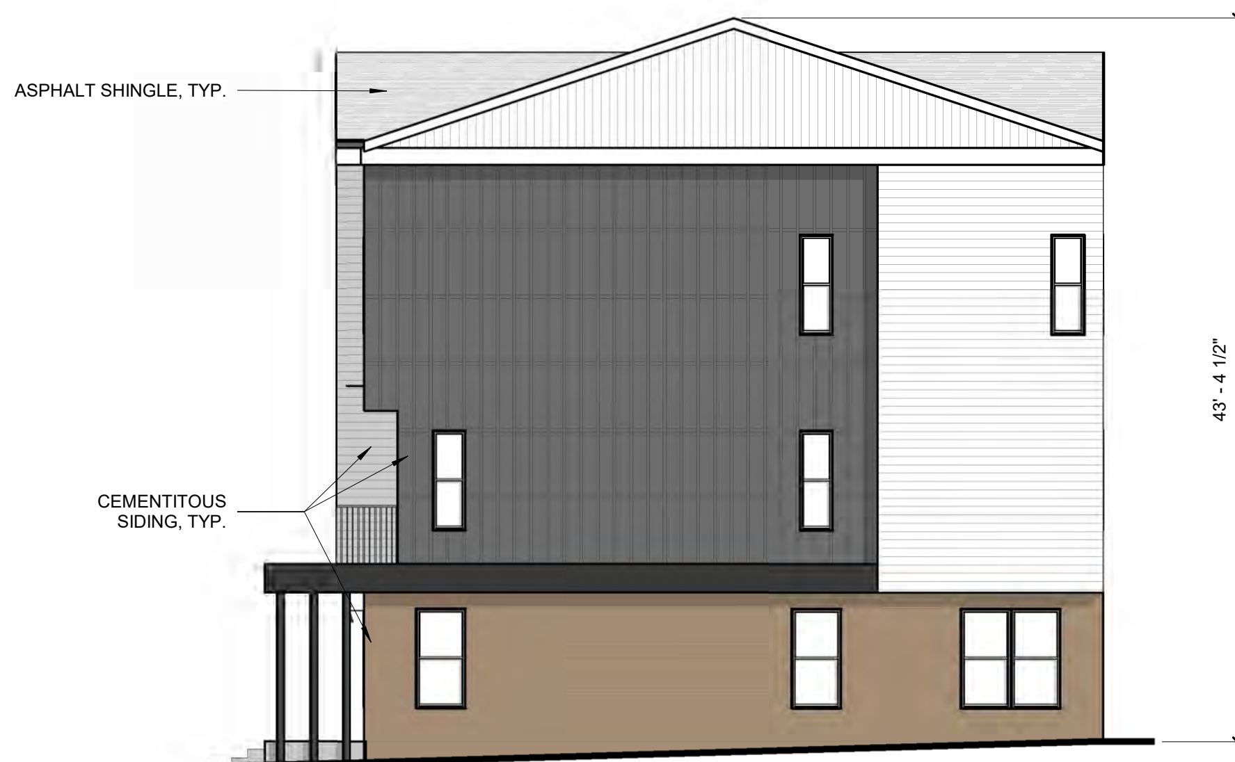
02 BUILDING A - RIGHT ELEVATION
