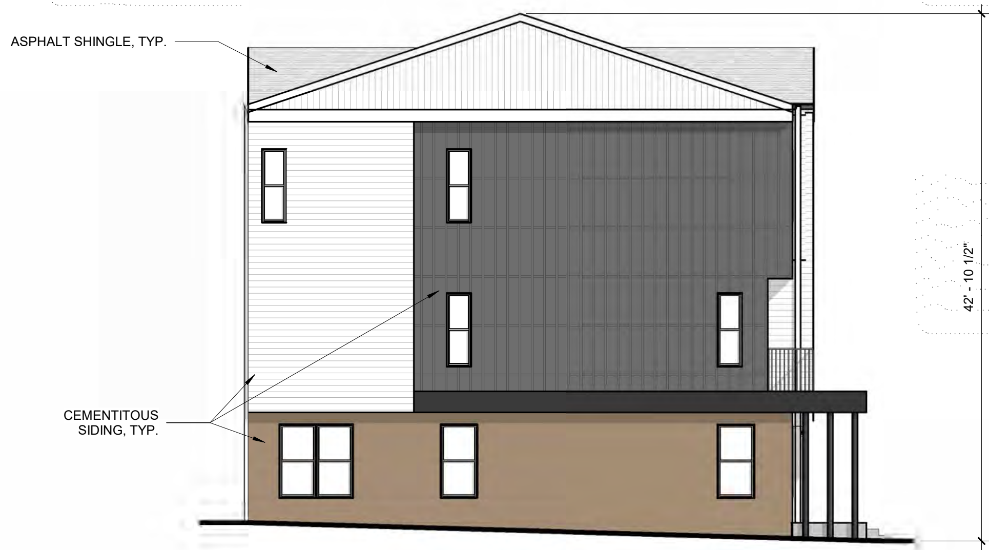
04 BUILDING A - LEFT ELEVATION
