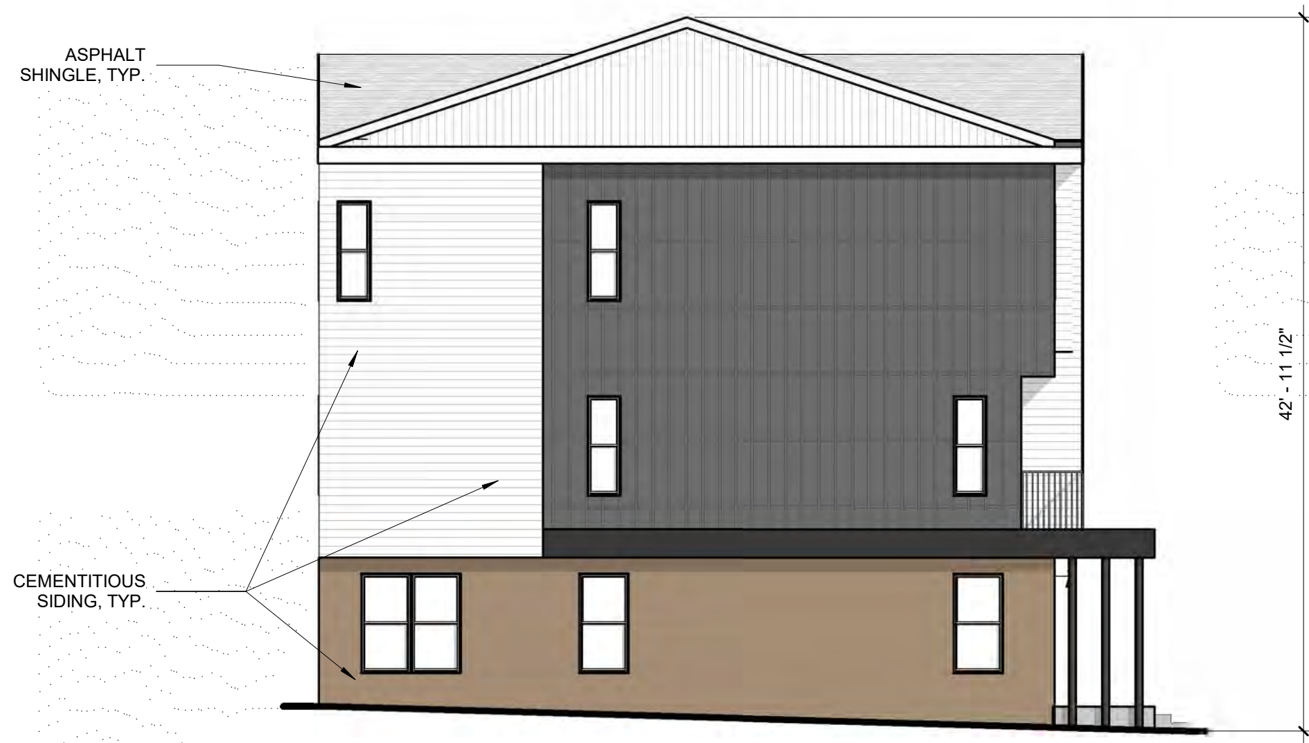
04 BUILDING H - RIGHT ELEVATION
