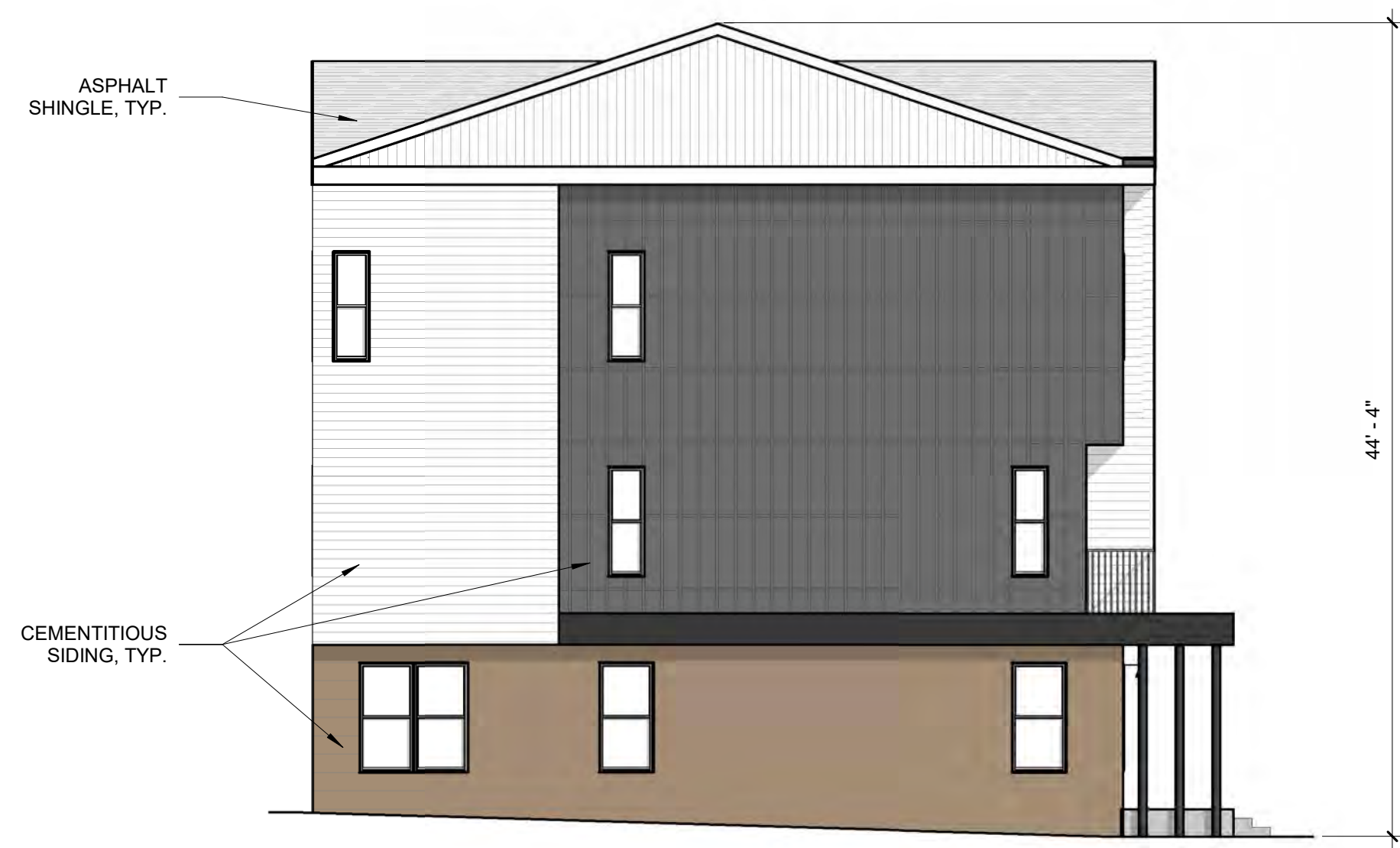
04 BUILDING G - LEFT ELEVATION
