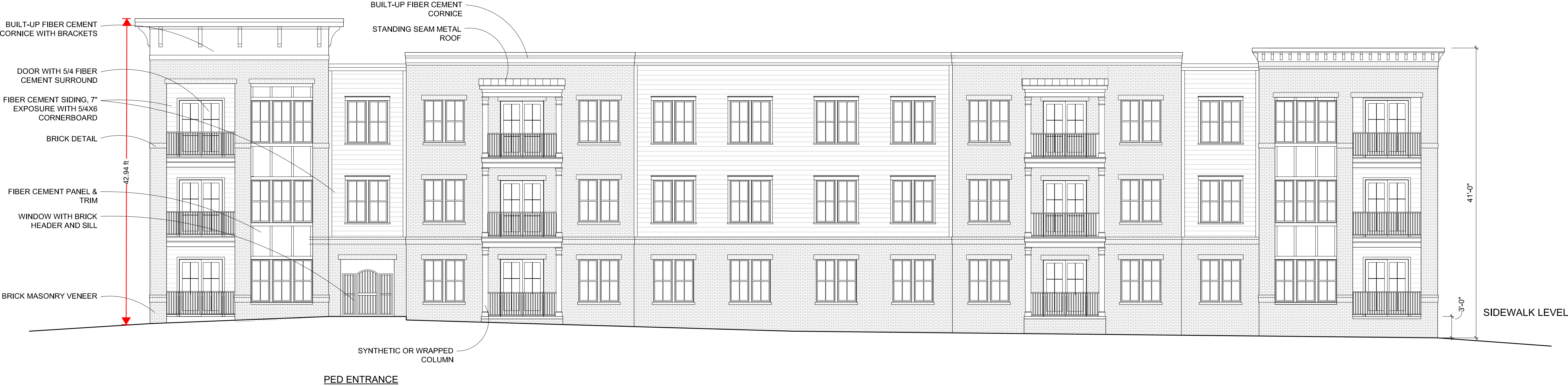
BUILDING 02 SIDEWALK ELEVATION - WEST
