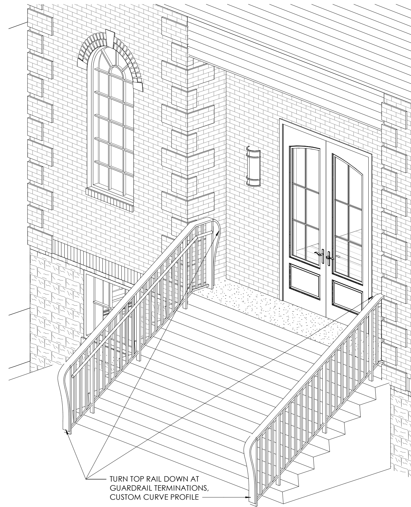
9 3D - ENTRY STAIR GUARDRAIL
