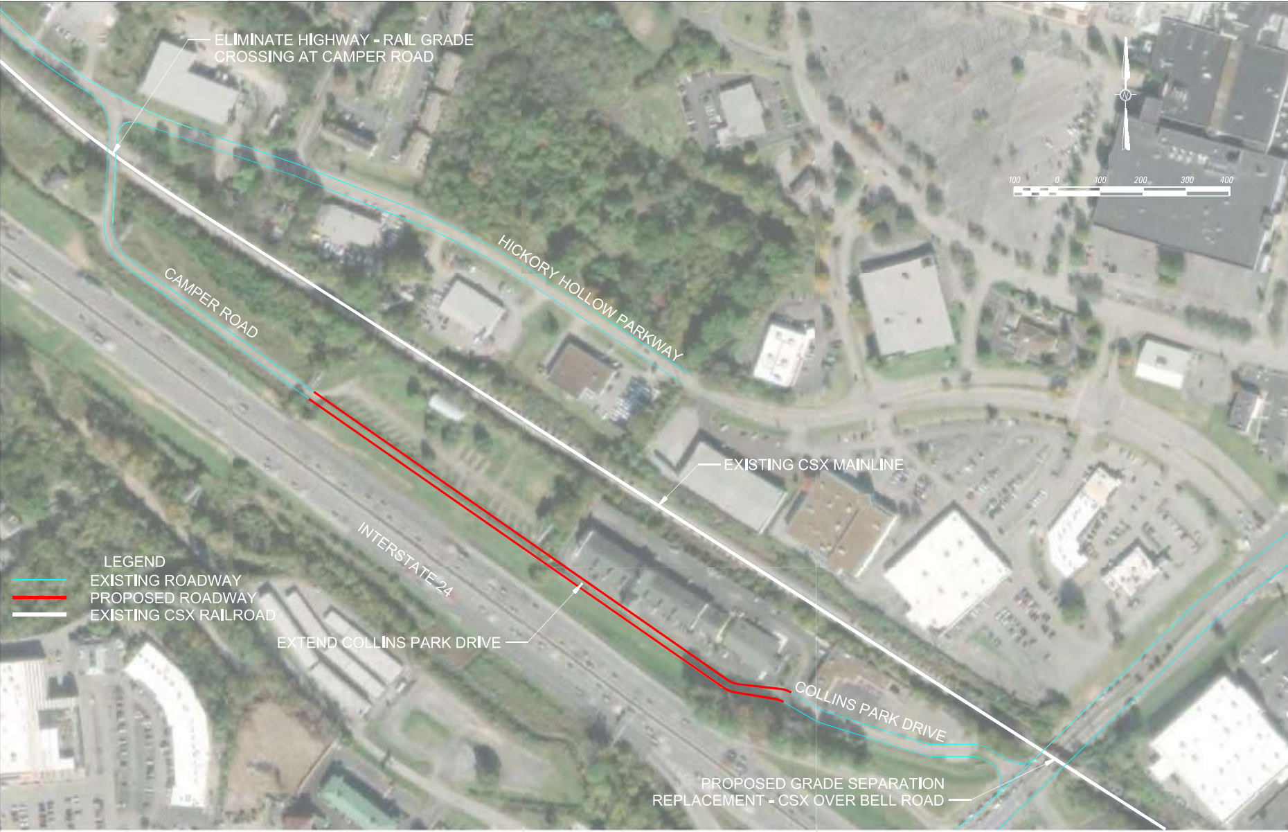
CAMPER ROAD GRADE CROSSING CLOSURE AND BELL ROAD GRADE SEPARATION REPLACEMENT
