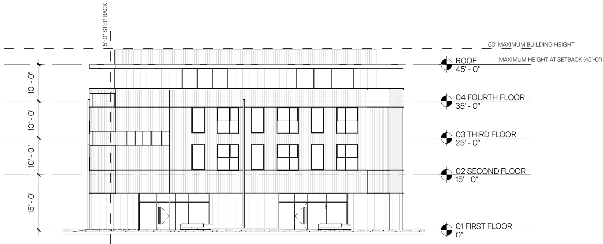
EAST ELEVATION FROM PILLOW ST SCALE: 1/16" = 1'
