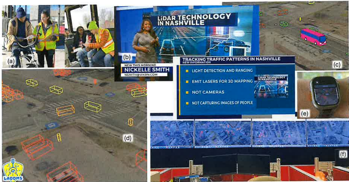
Figure 1. Overview of LADDMS Stage I results. (a) Community-centered engagement for vulnerable road users. (b) Emphasis on privacy and safety is disseminated through local media. (c) Automatic bus recognition within live viewing system for public transit integration. (d) Always-active live viewing system captures an impending near-miss (e) Mature data visualization tools operate in a browser as well as on mobile tech, such as a smart watch. (f) Live viewer deployment to the Nashville DOT Traffic Management Center (shown are 5 of the 7 sensor areas).
