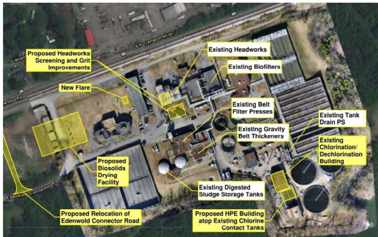
Figure 1-2. General Location Key for Proposed Improvements
