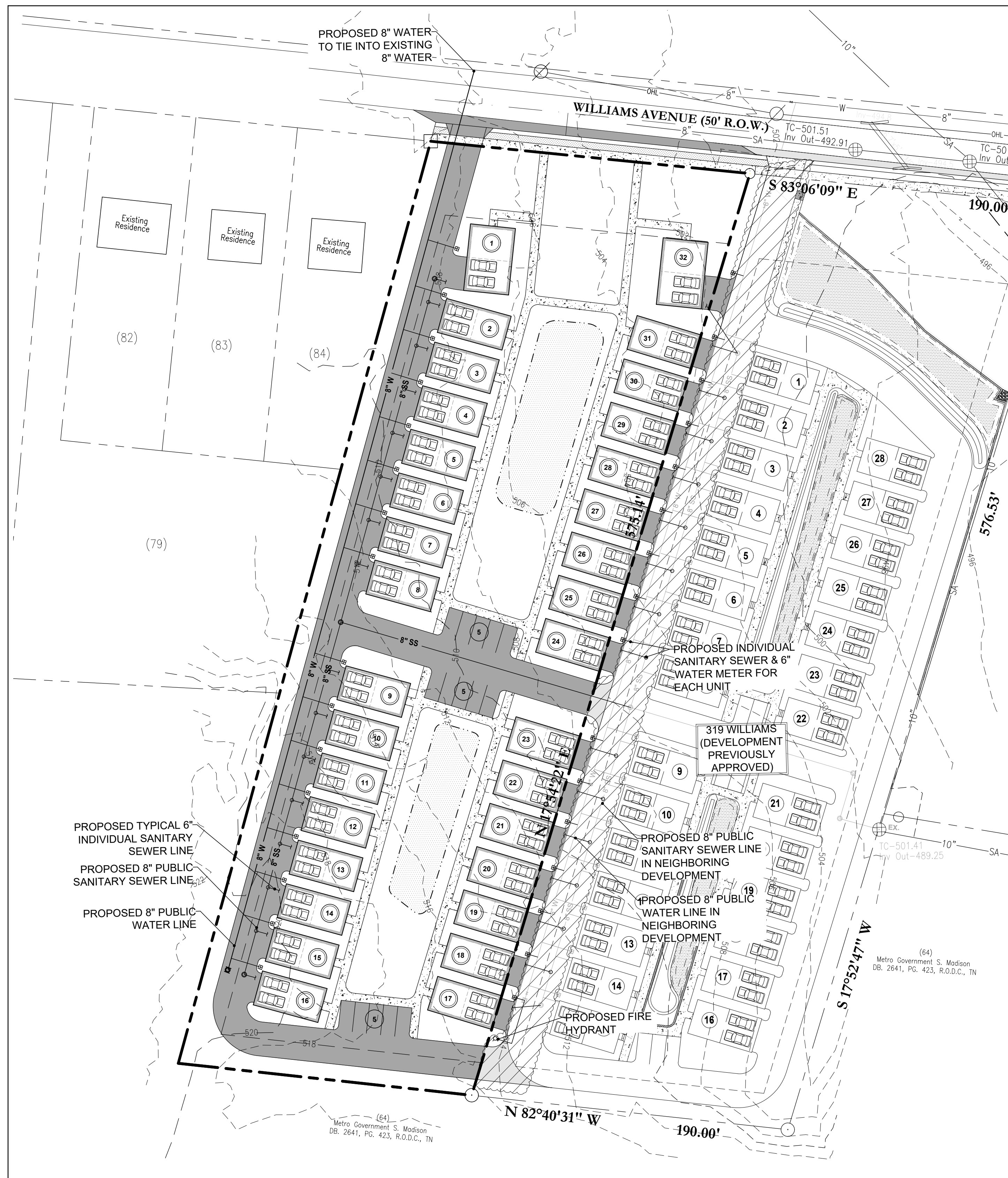
Utility and Grading & Drainage Plan (1"=40')
