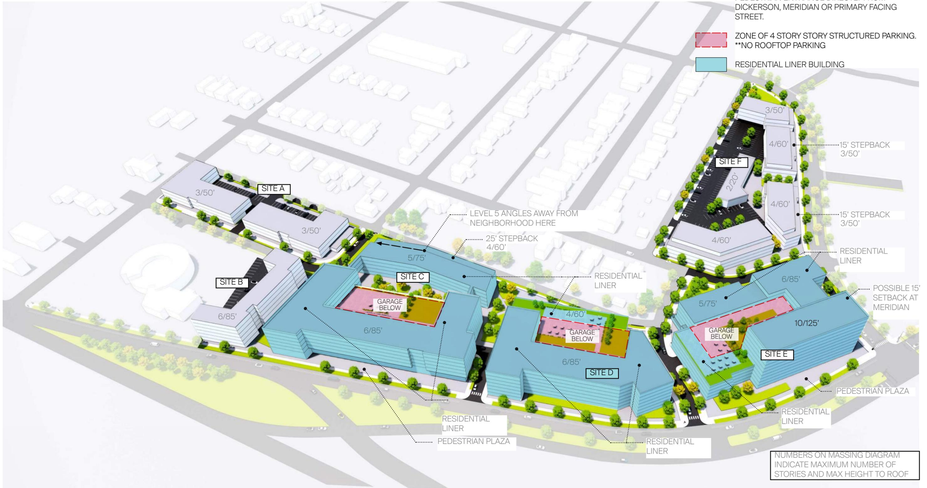
NUMBERS ON MASSING DIAGRAM INDICATE MAXIMUM NUMBER OF STORIES AND MAX HEIGHT TO ROOF
